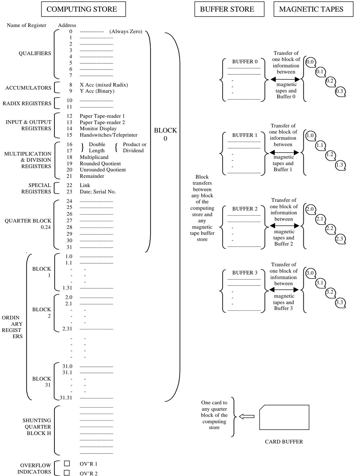
and manipulating and performing arithmetic on just that field, leaving the rest of the word unaffected. Such manipulations took place in the X-register, the Mixed Radix Accumulator. A binary accumulator was also provided, the Y-Register, for housekeeping within a program. The accumulators were part of the block of special registers (see Fig X2-9)
