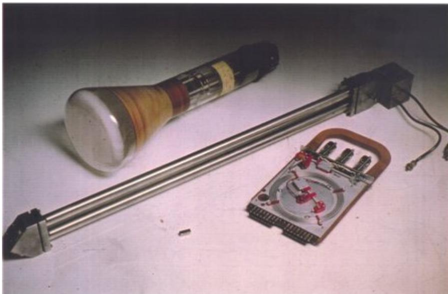
The upper left device in the photo is a CRT *Williams-Kilburn* storage tube from a Ferranti Mark I computer. In the centre is a mercury delay line from an English Electric DEUCE computer, where acoustic signals are transmitted down one tube and reflected back along
