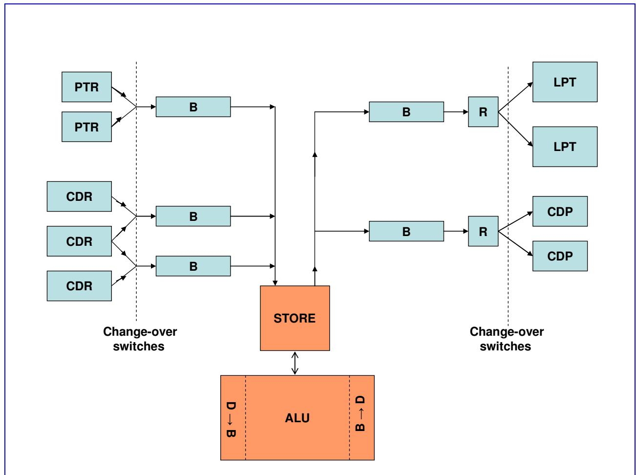
**Figure 2:** The three input and two output channels for LEO I.
