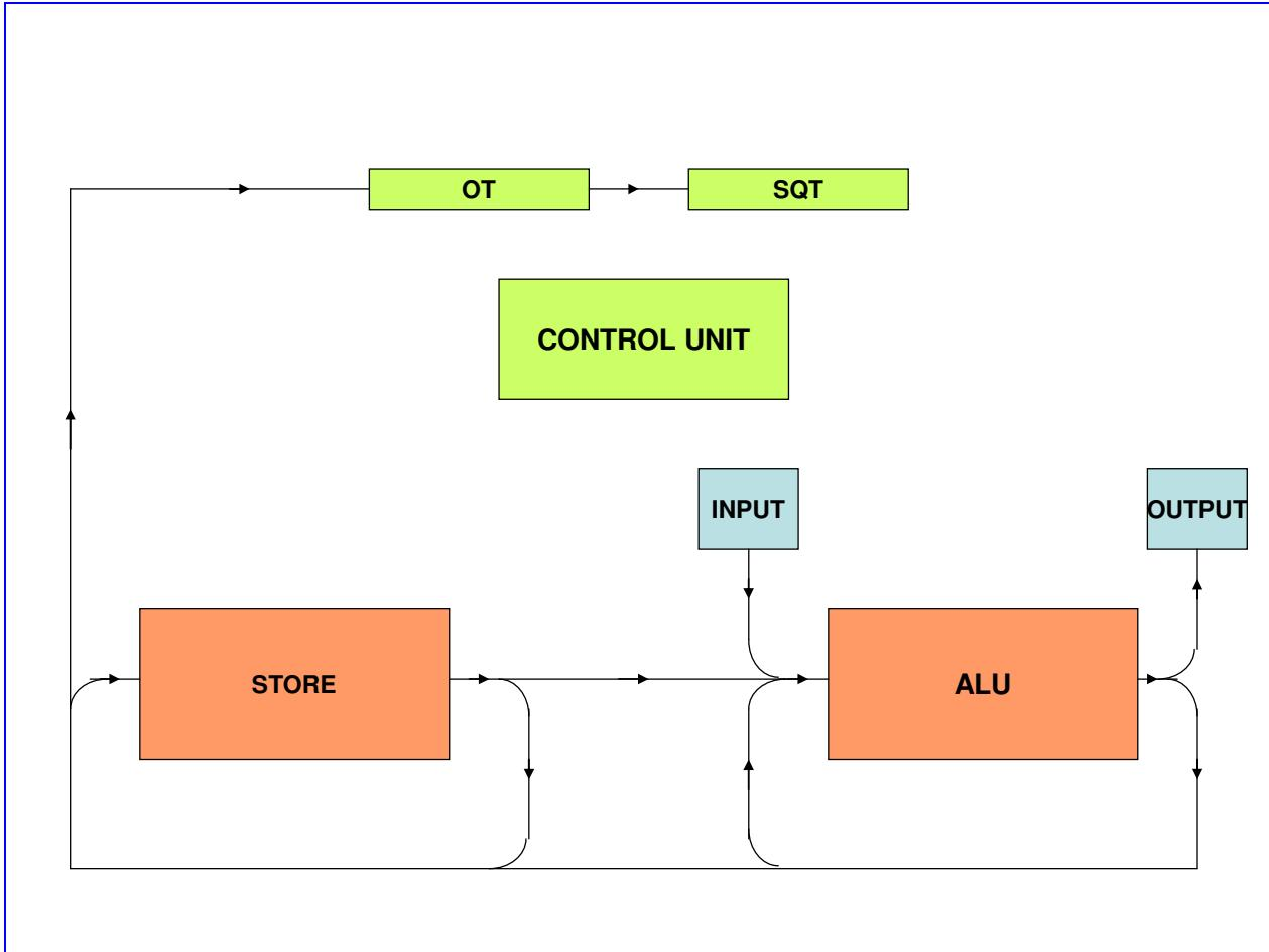
**Figure 1: simplified block diagram of EDSAC, showing the main information paths.**
