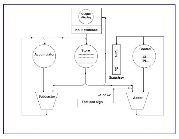
Figure 2.1. System diagram for the Manchester SSEM.
